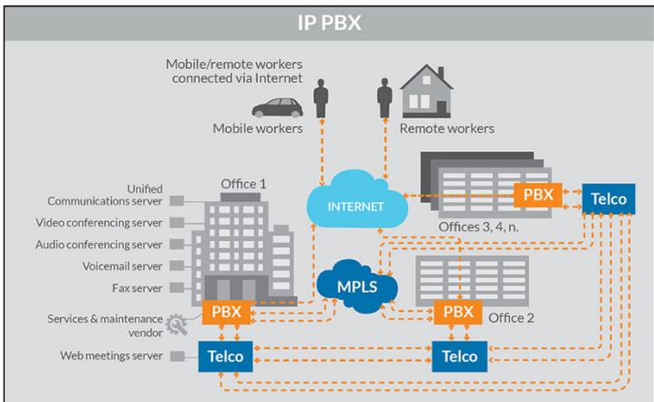
**FIGURE 1-2:** IP PBX systems enable converged networks and unified communications.
