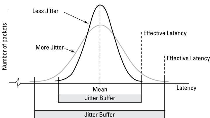
**FIGURE 4-1:** Jitter buffers can reduce jitter in VoIP calls.
