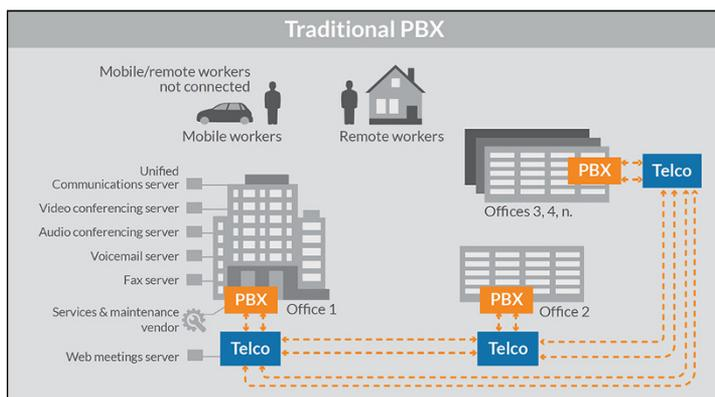
**FIGURE 1-1:** TDM PBXs provide limited integration with other apps and systems, and little or no support for mobile/remote workers.
